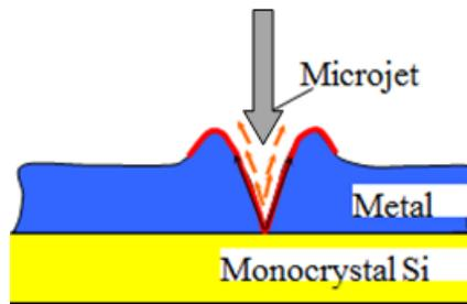
**Figure 36** Damage of a microchip in conditions SDP
