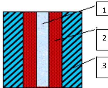
**Figure 28.** Scheme of canal zones: 1- "amorphous" or "nano" structure, 2- microstructure, 3- imperfect structure
