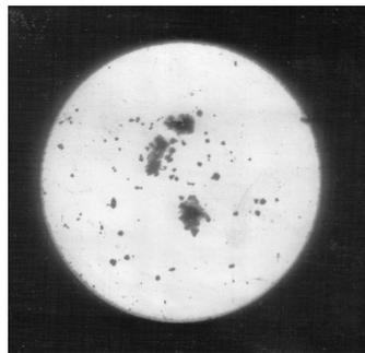
**Figure 22.** Radioautograph image of the steel 45 specimen on depth 4.3 mm dynamically alloyed by powdered particles W (C + <sup>14</sup>C) + Ni
