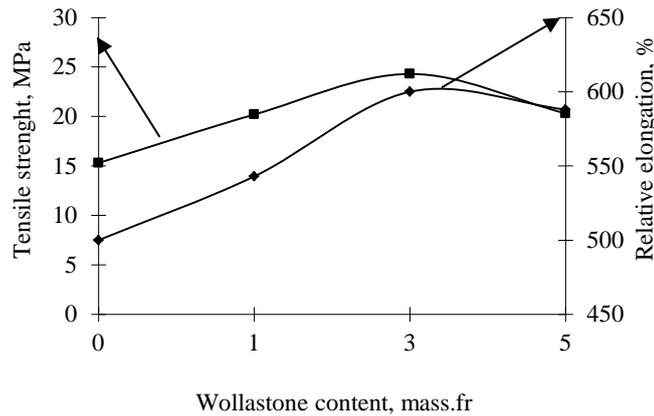
**Figure 43.** The concentration dependence of tensile strength and relative elongation of rubber mixtures based on isoprene elastomer.
