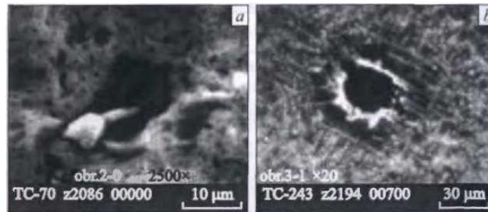
**Figure 38.** Tracks of damages in plastic films, received in a mode of superdeep penetrating, at processing in the protective container: (a) thickness of a barrier of 200 mm, 2 foil; (b) thickness of a barrier 50 mm, 31 foil
