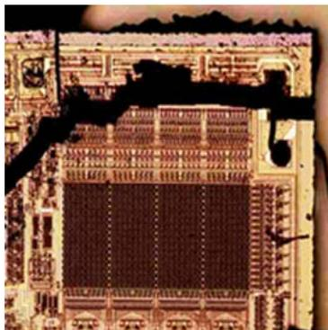
**Figure 33.** A view of the damaged monocrystal of silicon, x75
