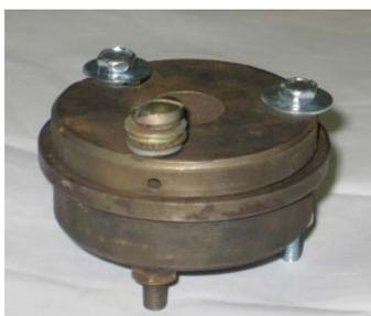
**Figure 41.** The container with rubber samples inside.
