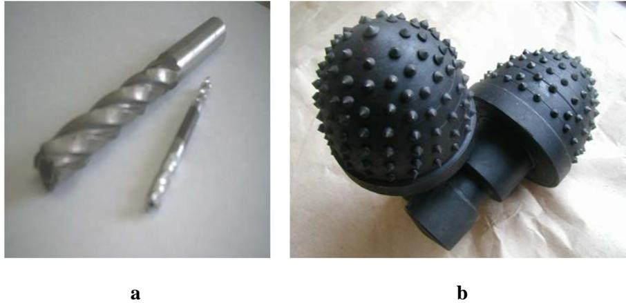
**Figure 24** Strengthen tools; **a-** Metal cutting tools ; **b-** The tools for cracking of coal
