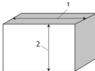
**Figure 31.** The scheme of measurement of electric resistance in composite material: **1-** along; **2-** across
