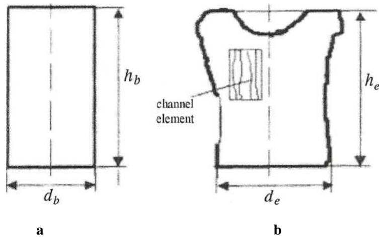
**Figure 5.** Changes in the metal barrier, arising as a result of its impact with a clot of particles: **a-** initial cylindrical barrier  $h_b, d_b$ ; **b-** the barrier after the dynamic loading ( $h_e, d_e$ )
