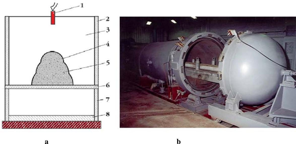
**Figure 19** a- The device for bursting alloying: 1-detonator; 2- metal bucket for explosive material; 3- charge of explosive material; 4- metal bucket for cumulative metal bucket for cone; 5- powder composition; 6-plate – bottom of cartridge; 7- regulative abutment; 8- barrier; b- Installation for SDP treatment
