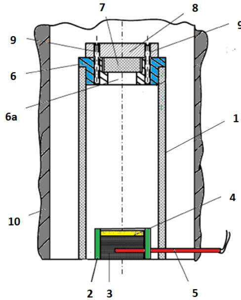
**Figure 46.** Vertical view of constructed device for membrane production by SDP method. **1-** tubular shell; **2-** cartridge; **3-** detonatable explosive material; **4-** supersaturated solution of water-soluble solid salt; **5-** detonator; **6-** membrane holder; **7-** cavity of the holder; **8-** cover of the holder; **9-** fasteners; **10-** explosion-proof chamber
