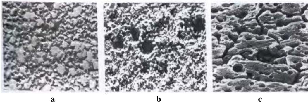
**Figure 12.** HSS steel at different stages of processing: **a** - before processing, x 1,000; **b** - after SDP, x 1,000; **c** - after SDP and heat treatment, x 5,000
