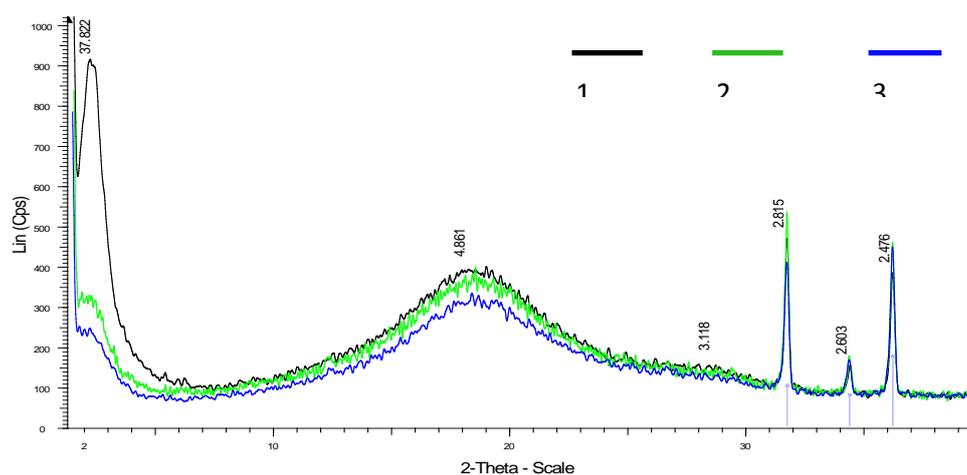
**Figure 42.** Diffractogram of rubber mixtures based on isoprene elastomer (1) and its composition with 1 (2) и 3 (3) mass.fr. MMT (X-ray method at diffractometer D8ADVANCE)
