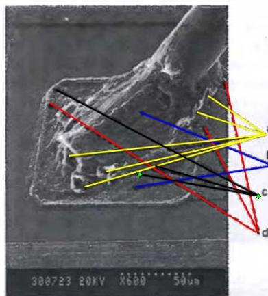
**Figure 37.** Features of interaction of a metal element of the microchipe with a plasma jet at SDP: **a** - zones of dynamic extrusion of metal micropipes (microexplosions); **b** - a zone with the removed electroplating; **c** - zones with microholes; **d** - zones of microcracks
