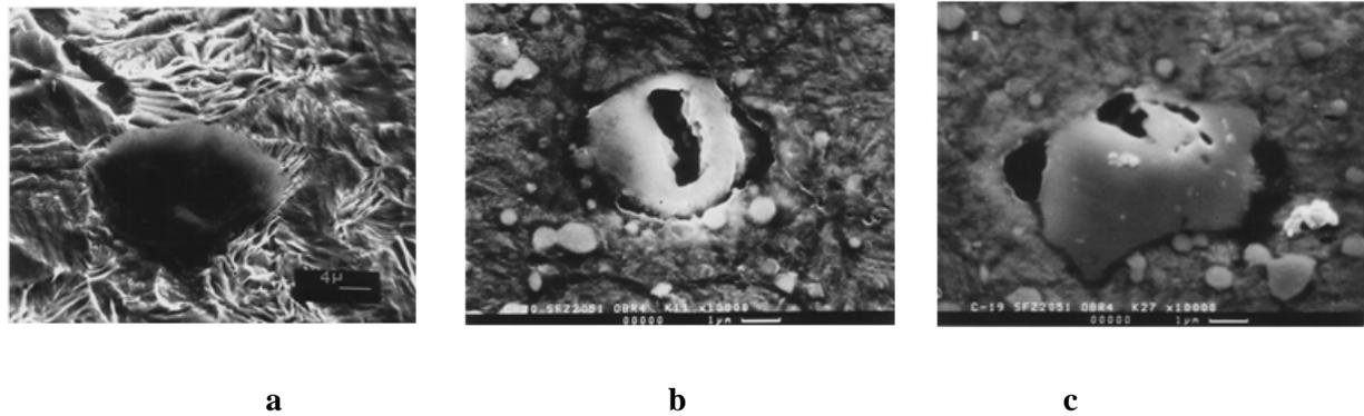
**Figure 13.** Zones of local fusion into HSS steel: **a** – x 2,200; **b,c** - x 10,000
