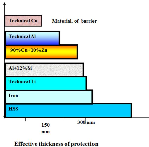
**Figure 20.** Penetration distance of a dust strikers depending on metal barrier
