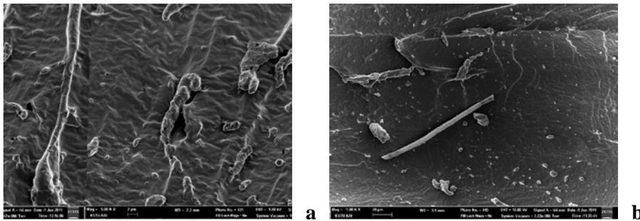
**Figure 44.** The scanning electronic microscope (Auriga device of Zeiss) pictures of structure of rubbers based on isoprene elastomer, modified with 3 mass. fr. of wollastone by SDP method (b) and mixing in melt (a)
