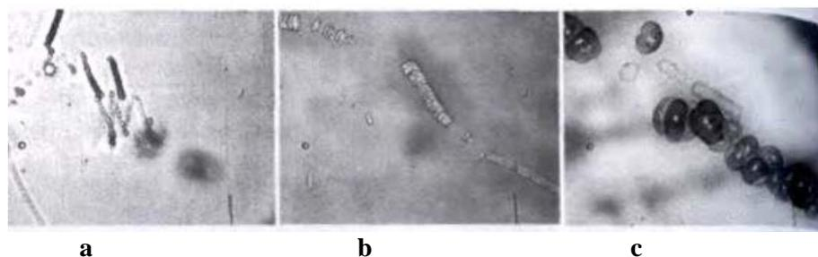
**Figure 45.** Structure processed in SDP mode of glass sample after various modes of etching x 1,000: (a) 30 s, (b) 60 s, (c) 120 s
