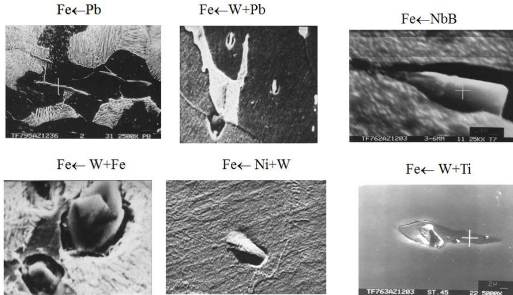
**Figure 8.** Microslices of the steel samples after SDP treatment by different kinds of strikers
