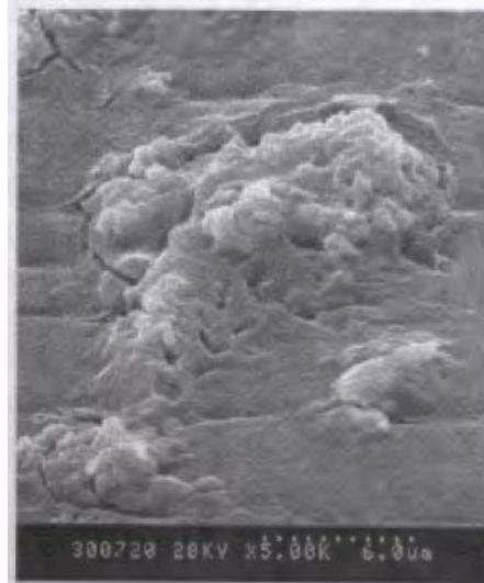
**Figure 34.** A zone of damage of a silicon plate in a soft mode
