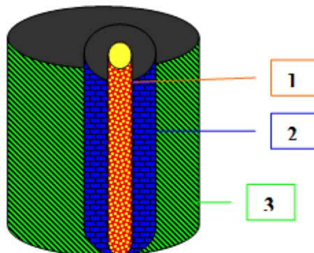
**Figure 6.** Scheme of a channel zone, **1** - amorphous material, **2** - microcrystalline material, **3** - defective material.
