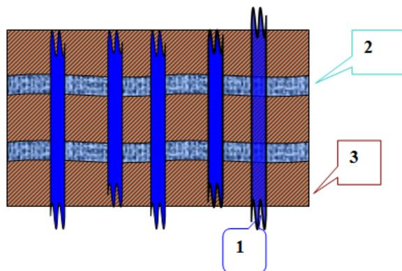
**Figure 29.** Scheme of structure of composite material: 1- zones of canals along to astir dust; 2- zone across to astir dust; 3- matrix material
