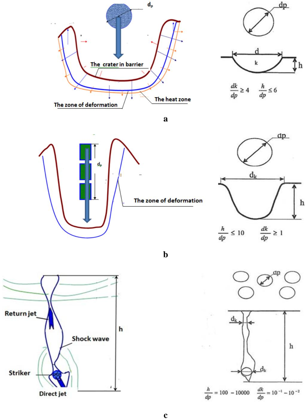
**Figure 1.** Comparison of characteristic features of various impacts with a barrier **a-** Usual; **b-** Anomalous; **c-** Superdeep penetration ,  $d_p$  - diameter of a striker,  $d_k$  - diameter of a crater, and  $h$  - crater depth
