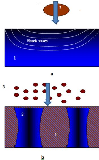
**Figure 10.** Formation macrozones of high pressure: **a** -Usual impact; 1- barrier; 2- striker; **b** – SDP impact; 1- zone of high pressure; 2- zone of low pressure; 3- disperse striker
