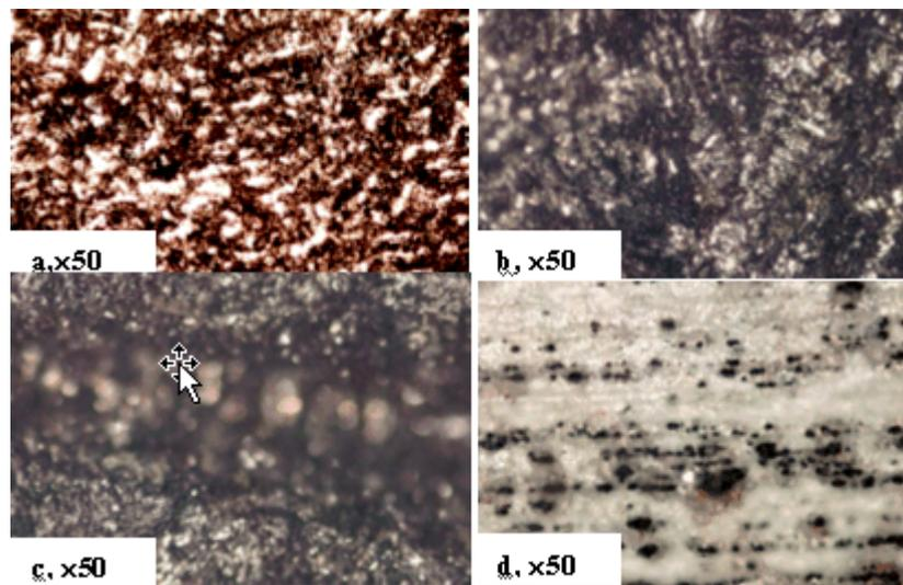
**Figure 25.** Structure of aluminum alloy Al+12%Si: **a** - after casting; **b** - without etching after SDP; **c** - after SDP - SiC and after electrochemical etching; **d** - after SDP-Pb and after electrochemical etching.
