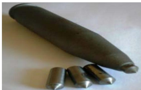
**Figure 23.** Self-sharpening mining tool and metal blocks from the composite tool material
