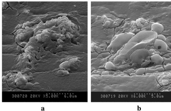
**Figure 35.** Segments of local melting on a surface of a silicon plate: **(a)** a zone of formation of melting; **(b)** a zone of initiation of growth of new monocrystals of silicon
