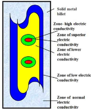
**Figure 30 .** Distribution of electric conductivity zones at impact
