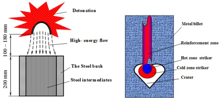
**Figure 18.** Schematic view illustrating penetration of the flow of working medium in the volume of a preform of initial tool steel for forming the composite steel material .
